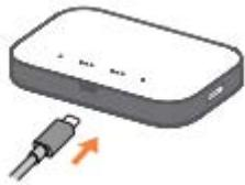
Charge using a charger and USB data cable. Connect the USB cable into the charging port as shown and connect the charger to a power outlet to start charging. When the device is powered off, it takes about 3 hours before being fully charged. Note: When red battery indicator lights up, device should be charged to protect the battery.
