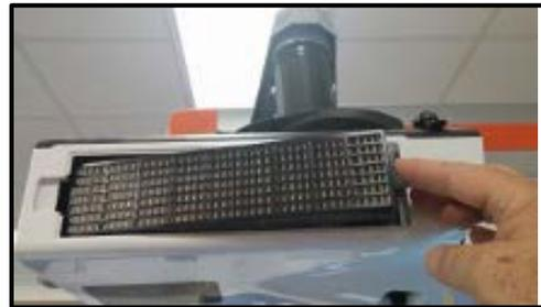
\*\*When taking out the filter, put your finger on the right side of the filter and pull it out.
