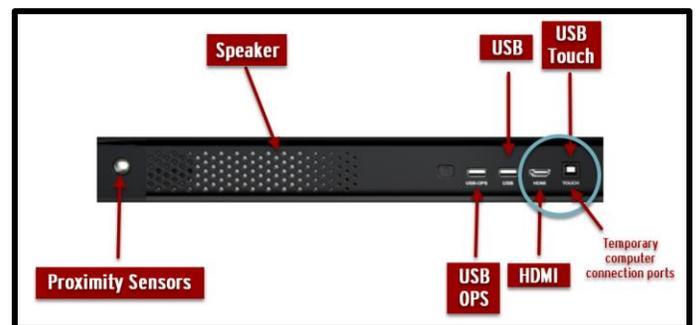
**PROXIMITY SENSORS:** The Proximity Sensors turn your panel on when you enter the room and will shut your panel down after 2 hours of inactivity.
